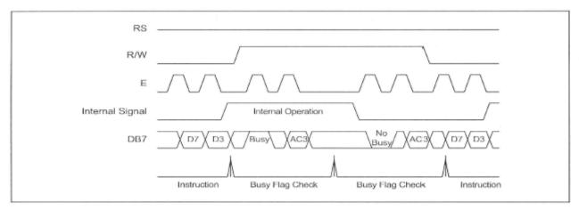
Example of 4-bit Bus Mode Timing Sequence
