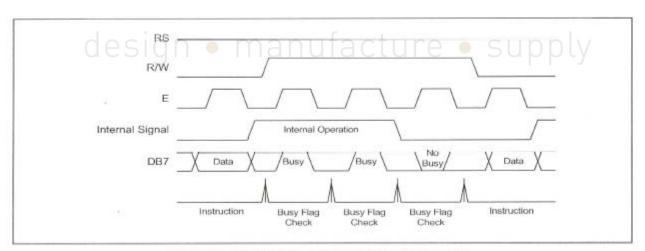
Example of 8-bit Bus Mode Timing Sequence
