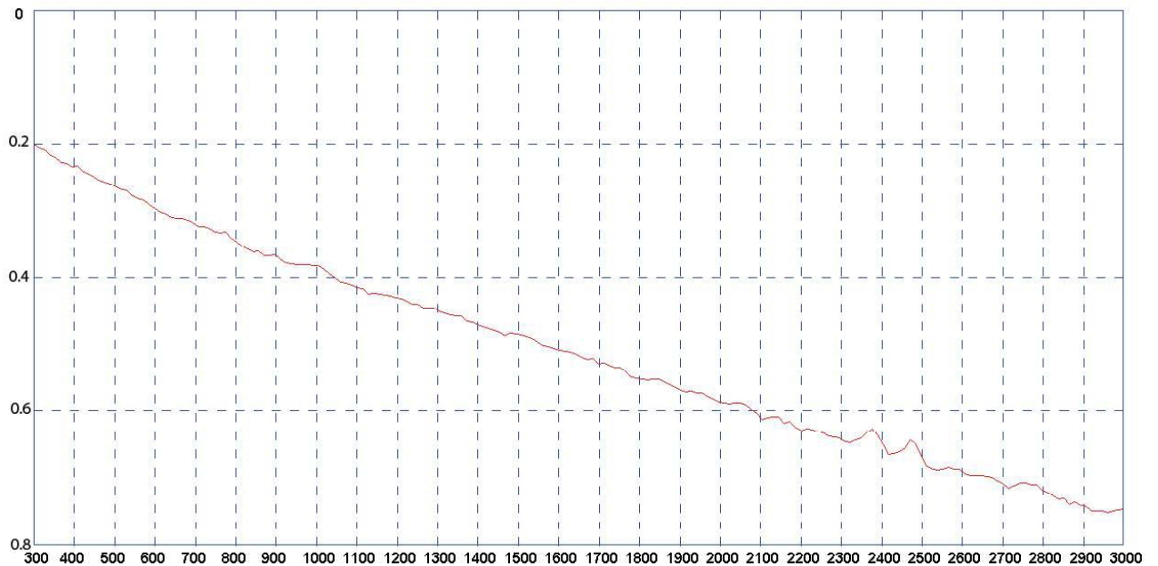
Typical Attenuation dB per m of Cable*
