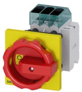
Load disconnector 3LD3, Iu 16 A Main switch 3-pole Rated operating capacity at AC-23 A at 400V 7.5kW Front plate mounting Basic switch with Central hole mounting 22.5mm Rotary actuator red / yellow 66 x 66 mm with auxiliary switch 10E + 1S
