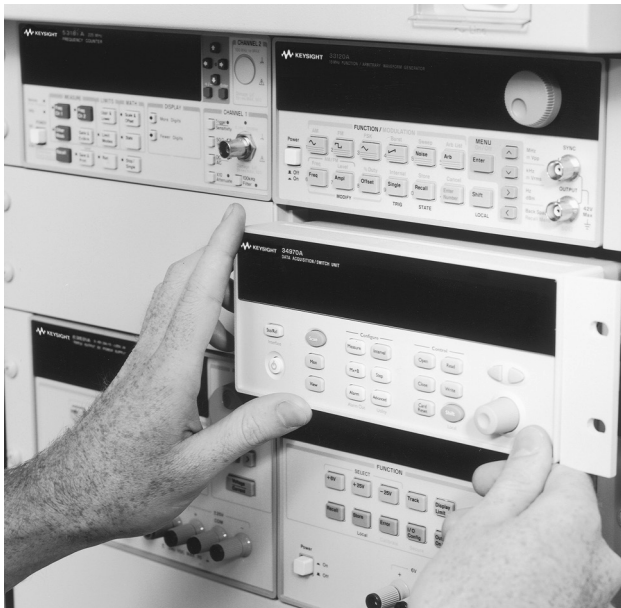
Low-cost switching system for automated testing
