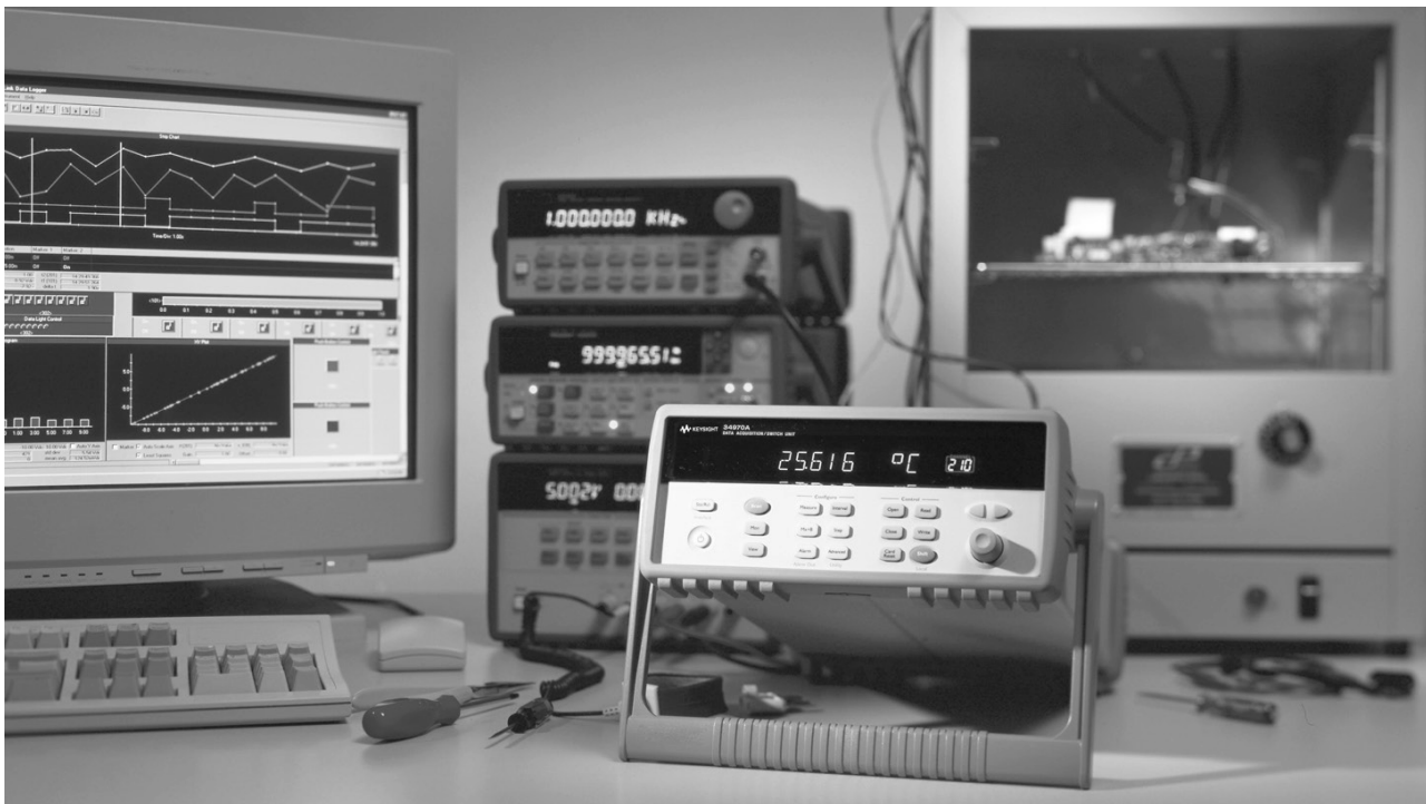
Compact 60-channel data acquisition system
