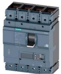
CIRCUIT BREAKER 3VA2 IEC FRAME 400 BREAKING CAPACITY CLASS M ICU=55KA @ 415 V 4-POLE, LINE PROTECTION ETU850, LSI, IN=400A OVERLOAD PROTECTION IR=160A ...400A SHORT CIRCUIT PROTECTION ISD=0,6..10X IN, II=1,5..10X IN NEUTRAL PROTECTION ADJUSTABLE (OFF, UPTO 100%) BUSBAR CONNECTION
