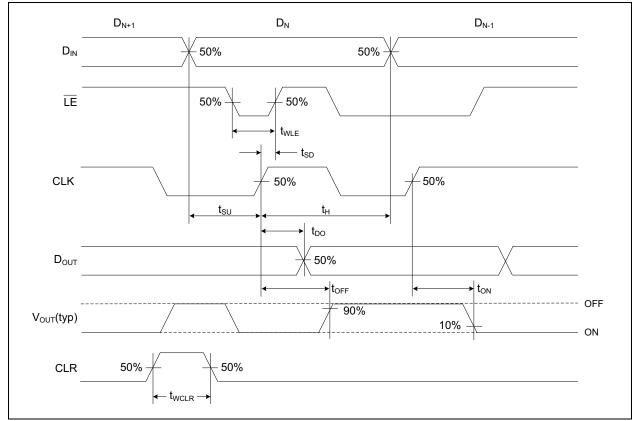
FIGURE 1-1: Logic Input Timing Diagram.
