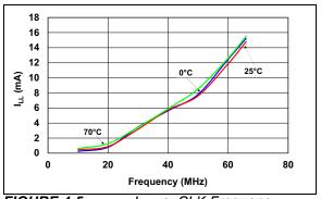
FIGURE 4-5: I<sub>LL</sub> vs. CLK Frequency.
