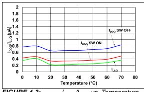
FIGURE 4-3: I<sub>DDQ</sub>/I<sub>LLQ</sub> vs. Temperature.
