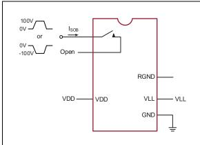
FIGURE 3-2: Switch Off Bias per Switch.
