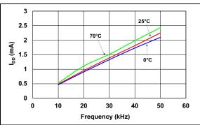
FIGURE 4-2: I<sub>DD</sub> vs. Switching Frequency.
