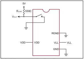
FIGURE 3-4: T<sub>ON</sub>/T<sub>OFF</sub> Test Circuit.
