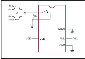
FIGURE 3-1: Switch Off Leakage per Switch.
