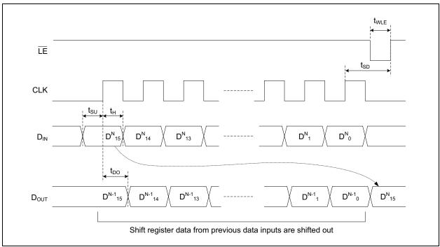
FIGURE 5-2: Latch Enable Timing Diagram.
