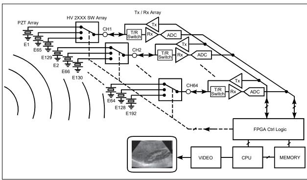
FIGURE 5-1: Typical Medical Ultrasound Imaging System.
