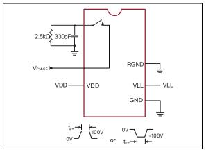
FIGURE 3-5: Tx Pulse Width.
