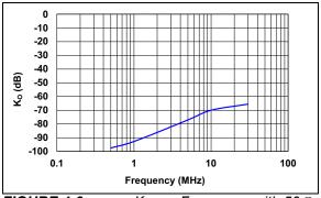
**FIGURE 4-6:**  $K_O$  vs. Frequency with  $50\Omega$  Load.
