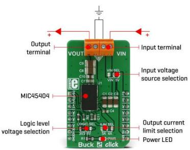
PWM switching frequency can be changed by the FREQ pin, routed to the PWM pin of the mikroBUS™ socket. The switching frequency is related to the selected output voltage and for this reason, it is routed to the mikroBUS™ socket, so that the voltage output and the corresponding frequency for the selected voltage can be set. There are three possible frequency values: 400kHz, 565kHz, and 790kHz.
