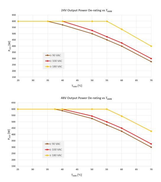
Figure 2. Power Derating Curves of MBS601 Series V1 Pout to TAMB
