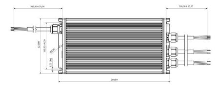
Figure 3. Mechanical drawing
