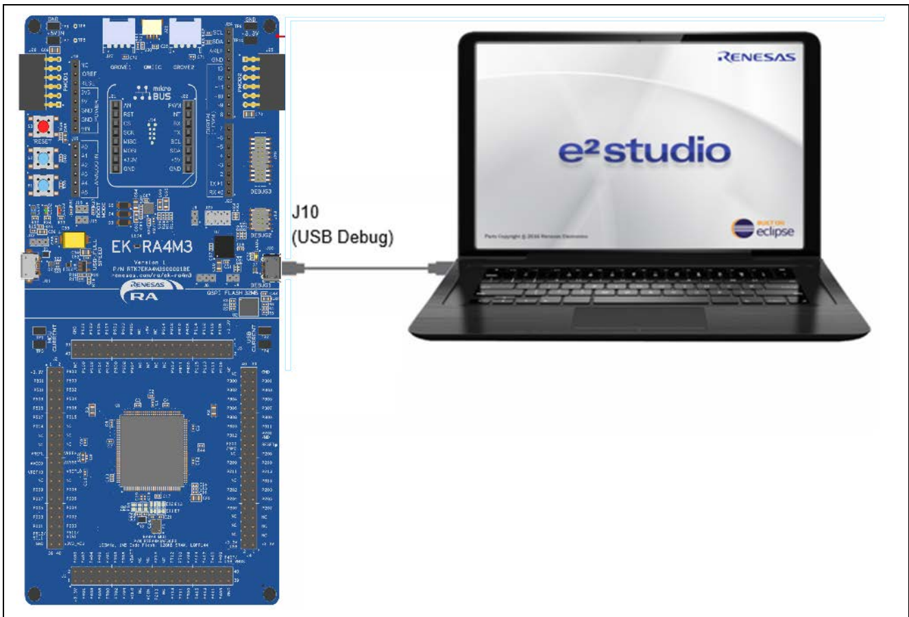
Figure 23. Connecting the EK-RA4M3 Board to the Host PC via USB Debug Port
