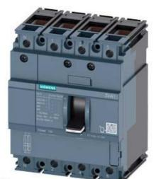
CIRCUIT BREAKER 3VA1 IEC FRAME 100 BREAKING CAPACITY CLASS N ICU=25KA @ 415 V 4-POLE, LINE PROTECTION TM210, FTFM, IN=80A OVERLOAD PROTECTION IR=80A FIXED SHORT CIRCUIT PROTECTION II=10 X IN NEUTRAL UNPROTECTED CABLE CONNECTION
