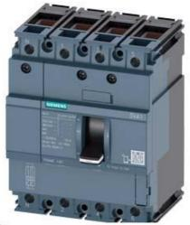
CIRCUIT BREAKER 3VA1 IEC FRAME 160 BREAKING CAPACITY CLASS N ICU=25KA @ 415 V 4-POLE, LINE PROTECTION TM210, FTFM, IN=25A OVERLOAD PROTECTION IR=25A FIXED SHORT CIRCUIT PROTECTION II=10 X IN NEUTRAL PROTECTION 100% CABLE CONNECTION
