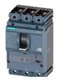
CIRCUIT BREAKER 3VA2 IEC FRAME 100 BREAKING CAPACITY CLASS L ICU=150KA @ 415 V 3POLE, LINE PROTECTION ETU330, LIG, IN=40A OVERLOAD PROTECTION IR=16A ...40A SHORT CIRCUIT PROTECTION II=1,5...12 X IN GROUNDFAULTPROTECTION IG=0,2... 1 X IN, TG=0,1/0,3MS BUSBAR CONNECTION
