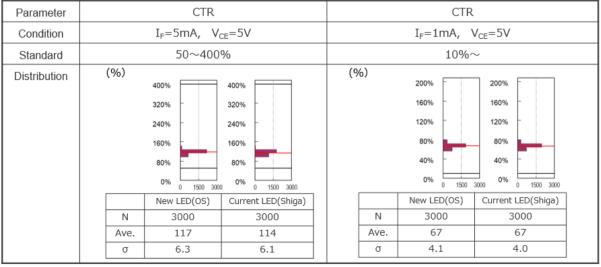
%Almost the same characteristic distribution is obtained before and after changing the LED.
