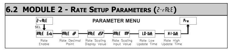
Module 2 is the programming for the Rate parameters. For maximum input frequency, Rate Enable should be set to MI when not in use. When set to MI, the remaining rate parameters are not accessible. The Rate value is shown with an annunciator of "" in the Display Mode.
