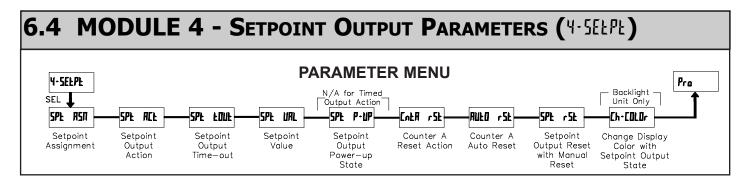
The Setpoint Output Parameters are only active when the optional relay module is installed in the meter. Some parameters will not appear depending on the Setpoint Assignment and Setpoint Output Action selected.
