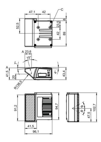
A Optical axis B Deflection angle of the laser beam:  $\pm$  30  $^{\circ}$  C M4 thread (5 deep)
