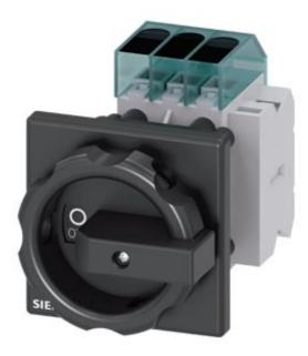
Switch disconnector 3LD3, main switch 3-polig, lu 32A operational switch at AC-23 A at 400 V 11,5 kW front mounted Base mounting with center-hole 22,5 mm rotary operationg mechanism black 66 x66 mm with auxiliary 1NO+1NC
