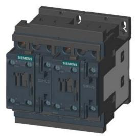
REV. COMB., AC3, 15KW/400V AC110V, 50/60HZ, 3-POLE, SZ S0 SCREW TERMINAL ELECTR. AND MECH. INTERLOCK 2NO INTEGR.
