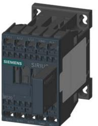
COUPLING RELAY, AC-3, 5.5KW/ 400V 1NO, DC 24V, 0.7...1.25\*US, W. PLUGGED-ON VARISTOR, 3-POLE SZ S00, SPRING-LOADED TERMINAL
