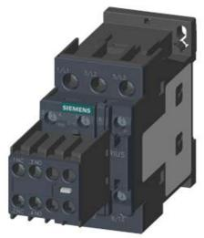
CONTACTOR, AC-3, 15KW/400V, 2NO+2NC, AC 24V 50HZ, 3-POLE, SZ S0 SCREW TERMINAL REMOVABLE AUX. SWITCH
