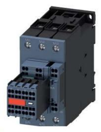
CONTACTOR,AC3:37KW/400V, 2NO+2NC, 230V AC 50/60HZ, WITH PLUGGED-IN VARISTOR, 3-POLE, SIZE S2, SPRING-TYPE TERMINAL, AUXILIARY CONTACT INSEPARABLE
