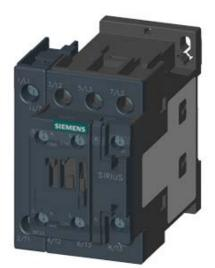
4NO CONTACTOR, AC1: 40A AC 230V 50HZ 4-POLE, 4NO, SZ: S0, SCREW TERMINAL 1NO+1NC INTEGR.
