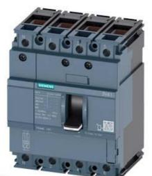
CIRCUIT BREAKER 3VA1 IEC FRAME 160 BREAKING CAPACITY CLASS S ICU=36KA @ 415 V 4-POLE, LINE PROTECTION TM210, FTFM, IN=40A OVERLOAD PROTECTION IR=40A FIXED SHORT CIRCUIT PROTECTION II=10 X IN NEUTRAL PROTECTION 100% CABLE CONNECTION
