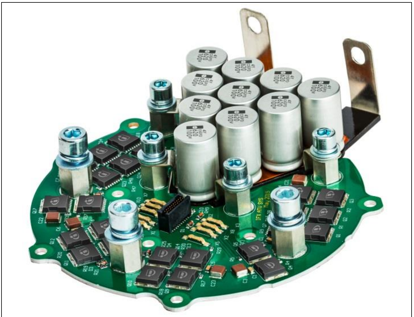
Figure 1 Overview of the power stage
