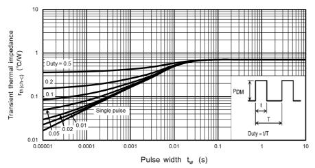
Fig. 8.13 r<sub>th</sub> - t<sub>w</sub> (Guaranteed Maximum)
