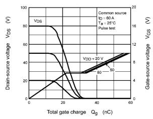
Fig. 8.10 Dynamic Input/Output Characteristics
