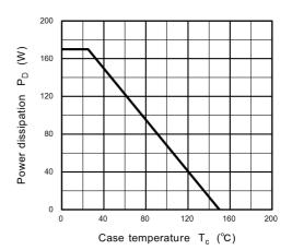
Fig. 8.15 P<sub>D</sub> - T<sub>c</sub> (Guaranteed Maximum)
