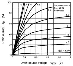
Fig. 8.2  $I_D - V_{DS}$
