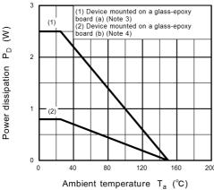
Fig. 8.14 P<sub>D</sub> - T<sub>a</sub> (Guaranteed Maximum)
