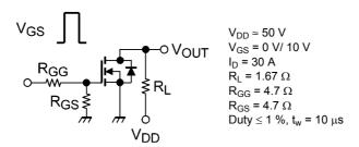
Fig. 6.2.1 Switching Time Test Circuit
