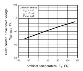
Fig. 8.7 V<sub>(BR)DSS</sub> - T<sub>a</sub>
