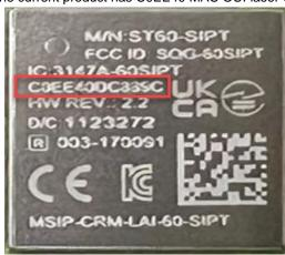
After this PCN, the product will have B0FB15 MAC OUI laser-etched on the RF shield and embedded in the barcode.
