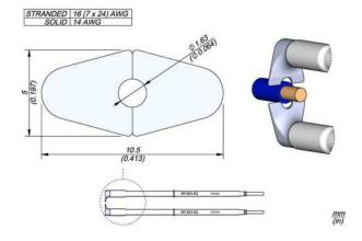
W14014G is specially designed for stripping high-temperature wire insulations made of thermostable materials such as Teflon\*, Kapton\*, silicone rubber, etc, of 14 AWG (1.63 mm / 0.0642 in).
