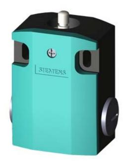
BASIC SWITCH FOR POSITION SWITCH 3SE51, METAL ENCLOSURE 56MM, DEVICE CONNECTION 3X(M20X1.5), 1NO/1NC SNAP-ACTION CONTACTS W/O ACTUATOR HEAD
