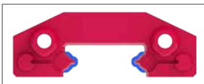
Smooth-running wiper (AL) (blue contour = contact surface)
