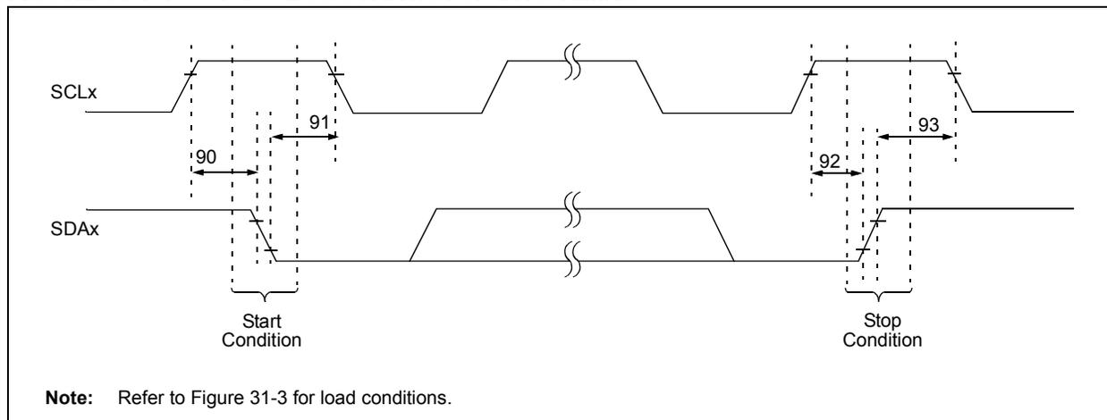
**TABLE 31-18: I<sup>2</sup>C™ BUS START/STOP BITS REQUIREMENTS (SLAVE MODE)**
