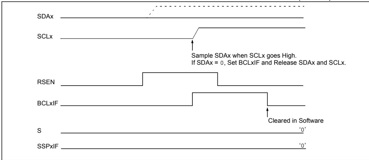
**FIGURE 21-32: BUS COLLISION DURING REPEATED START CONDITION (CASE 2)**
