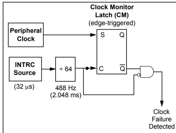
Clock failure is tested for on the falling edge of the sample clock. If a sample clock falling edge occurs while CM is still set, a clock failure has been detected (Figure 28-5). This causes the following:
