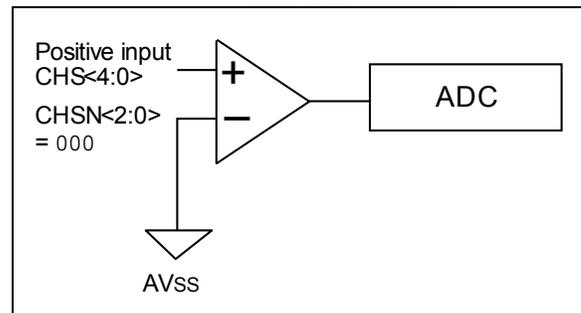
In the Single Channel Measurement mode, the negative input is connected to AVSS by clearing the CHSN bits (ADCON1<2:0>).
