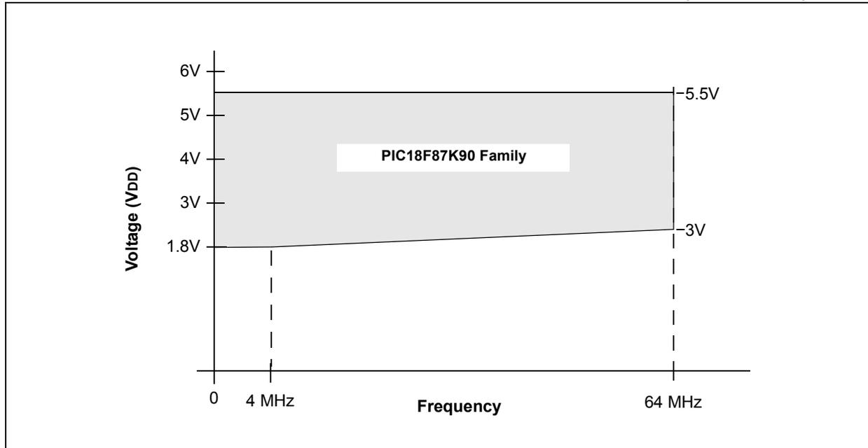
FIGURE 31-2: VOLTAGE-FREQUENCY GRAPH, REGULATOR DISABLED (INDUSTRIAL)<sup>(1,2)</sup>
