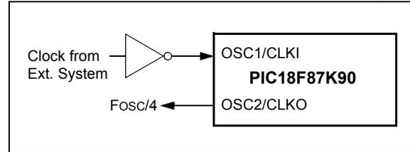
An external clock source may also be connected to the OSC1 pin in the HS mode, as shown in Figure 3-6. In this configuration, the divide-by-4 output on OSC2 is not available. Current consumption in this configuration will be somewhat higher than EC mode, as the internal oscillator's feedback circuitry will be enabled (in EC mode, the feedback circuit is disabled).
