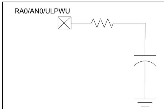
A timer can be used to measure the charge time and discharge time of the capacitor. The charge time can then be adjusted to provide the desired delay in Sleep. This technique compensates for the affects of temperature, voltage and component accuracy. The peripheral can also be configured as a simple programmable Low-Voltage Detect (LVD) or temperature sensor.
