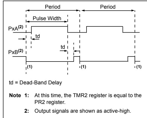
**FIGURE 19-15: EXAMPLE OF HALF-BRIDGE APPLICATIONS**
