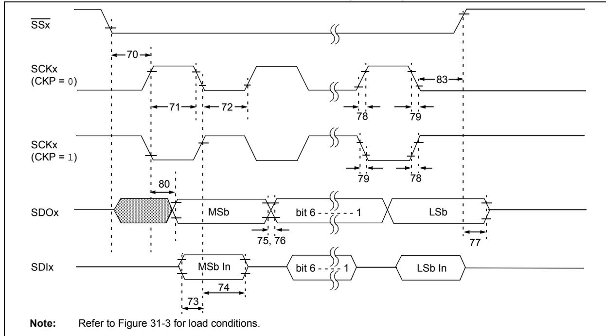
**TABLE 31-16: EXAMPLE SPI MODE REQUIREMENTS (SLAVE MODE TIMING, CKE = 0)**
