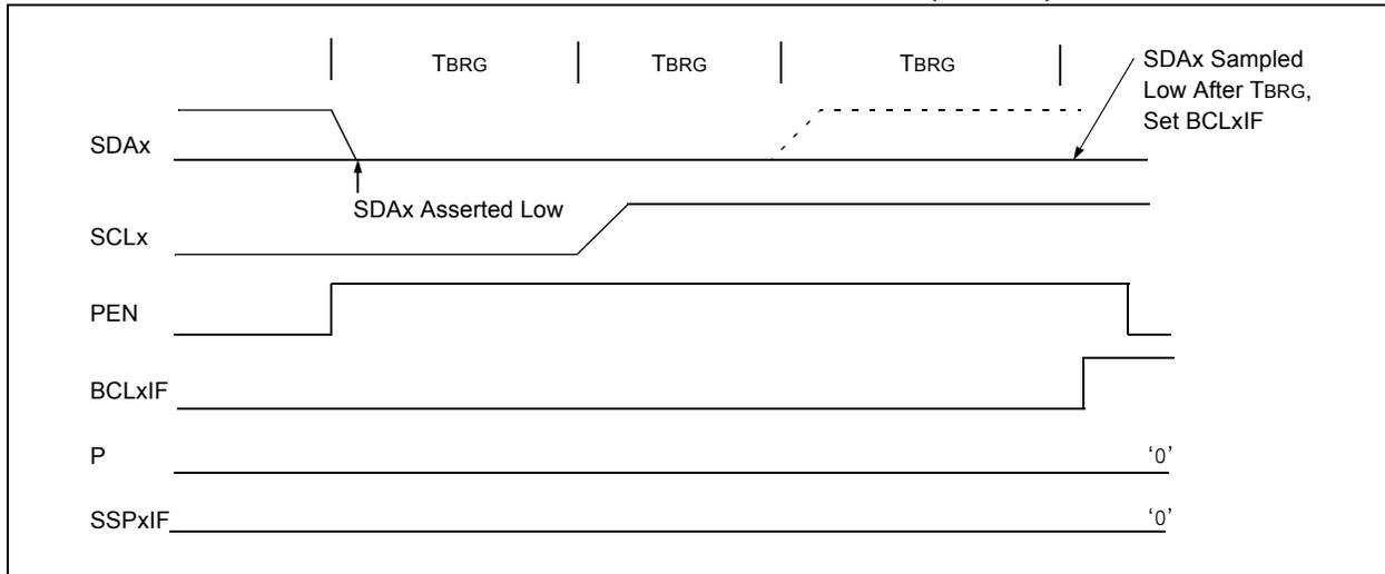
**FIGURE 21-34: BUS COLLISION DURING A STOP CONDITION (CASE 2)**
