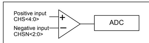
Differential conversion feeds the two input channels to a unity gain differential amplifier. The positive channel input is selected using the CHS bits (ADCON0<6:2>) and the negative channel input is selected using the CHSN bits (ADCON1<2:0>).
