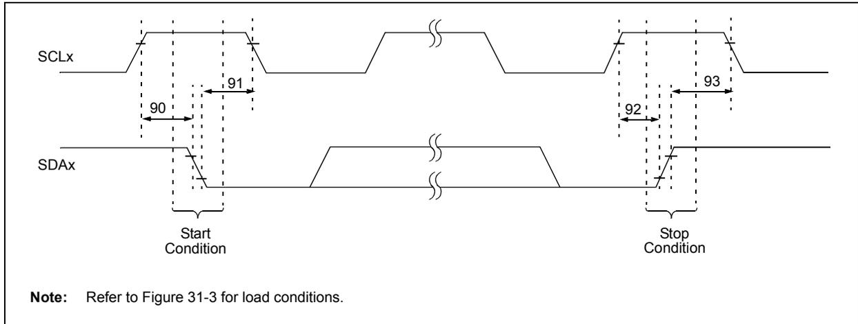
**TABLE 31-20: MSSP I<sup>2</sup>C™ BUS START/STOP BITS REQUIREMENTS**
