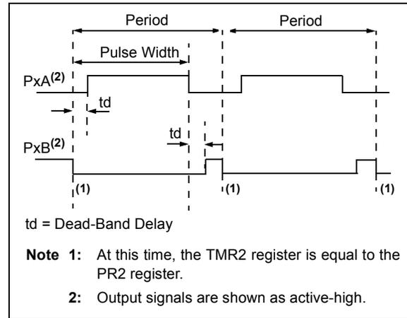
**FIGURE 19-7: EXAMPLE OF HALF-BRIDGE APPLICATIONS**
