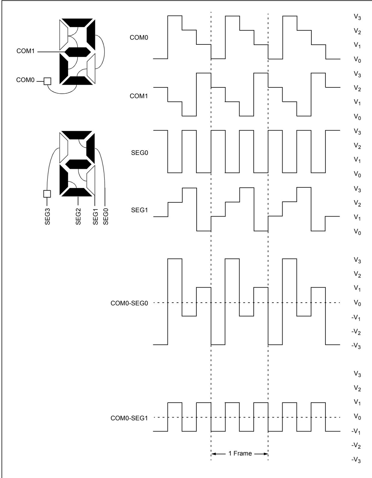
**FIGURE 20-11: TYPE-B WAVEFORMS IN 1/2 MUX, 1/3 BIAS DRIVE**
