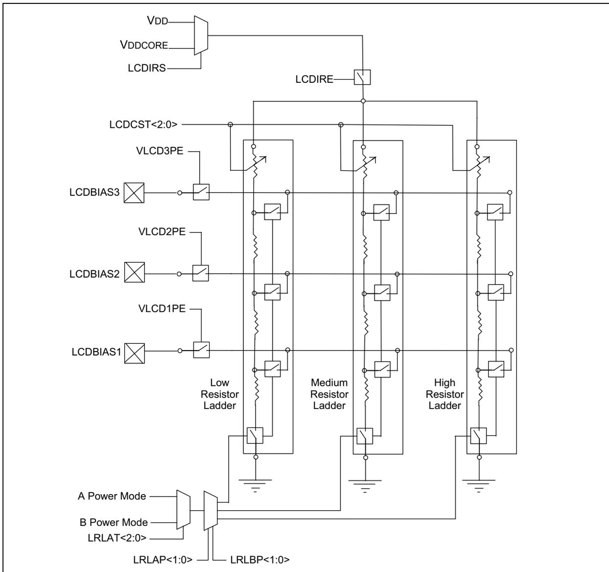
There are two power modes designated as “Mode A” and “Mode B”. Mode A is set by the bits, LRLAP<1:0> and Mode B by LRLB<1:0>. The resistor ladder to use for Modes A and B are selected by the bits, LRLAP<1:0> and LRLBP<1:0>, respectively
