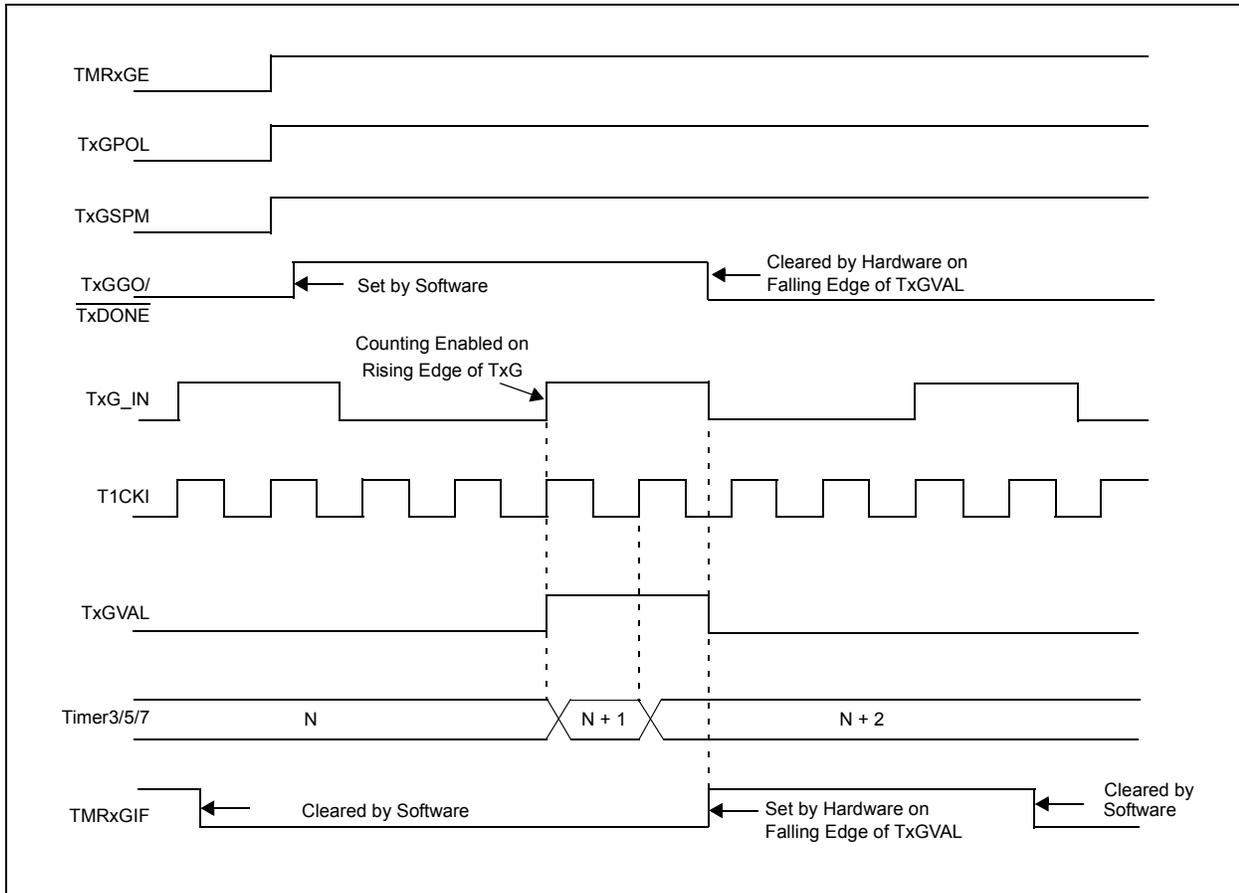
**FIGURE 15-5: TIMER3/5/7 GATE SINGLE PULSE AND TOGGLE COMBINED MODE**
