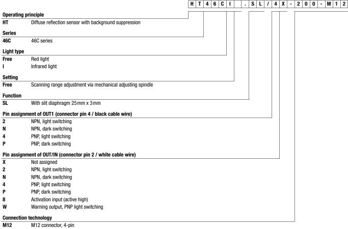
200-M12 Cable 200 mm with M12 connector, 4-pin
