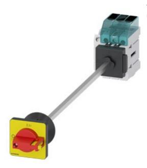
Switch disconnector 3LD3, main switch 3-polig, lu 16A operational switch at AC-23 A at 400 V 7,5 kW floor mounting Base mounting with door coupling center-hole 22,5 mm knob-operated mechanism red/yellow  $48 \times 48$  mm with auxiliary 1NO+1NC
