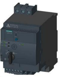
SIRIUS, COMPACT STARTER, REVERSING STARTER 690 V, 24 V AC/DC, 50 ... 60 HZ, 1 ... 4 A, IP20, MAIN CIRCUIT CONNECTION: SCREW TERMINAL, AUXILIARY CIRCUIT CONNECTION: SCREW TERMINAL
