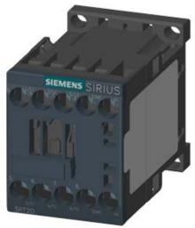
CONTACTOR, AC-3, 5.5KW/400V, 1NC, AC 230V, 50/60 HZ, 3-POLE, SZ S00 SCREW TERMINAL
