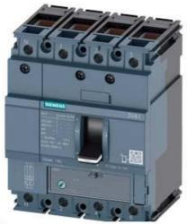
CIRCUIT BREAKER 3VA1 IEC FRAME 160 BREAKING CAPACITY CLASS N ICU=25KA @ 415 V 4-POLE, LINE PROTECTION TM220, ATFM, IN=25A OVERLOAD PROTECTION IR=17,5A ...25A SHORT CIRCUIT PROTECTION II=10 X IN NEUTRAL PROTECTION 100% CABLE CONNECTION
