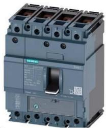
CIRCUIT BREAKER 3VA1 IEC FRAME 160 BREAKING CAPACITY CLASS N ICU=25KA @ 415 V 4-POLE, LINE PROTECTION TM220, ATFM, IN=40A OVERLOAD PROTECTION IR=28A ...40A SHORT CIRCUIT PROTECTION II=10 X IN NEUTRAL UNPROTECTED BUSBAR CONNECTION
