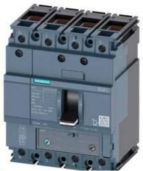
CIRCUIT BREAKER 3VA1 IEC FRAME 160 BREAKING CAPACITY CLASS N ICU=25KA @ 415 V 4-POLE, LINE PROTECTION TM240, ATAM, IN=63A OVERLOAD PROTECTION IR=44,1A ...63A SHORT CIRCUIT PROTECTION II=5...10 X IN NEUTRAL PROTECTION 100% CABLE CONNECTION
