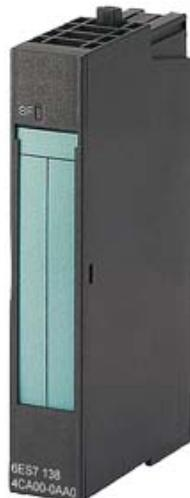
SIMATIC DP, ELECTRONIC MODULE ET 200S: 2AI RTD HIGH FEATURE, 15 MM WIDTH, 15BIT + SIGN ACCURACY +/- 0.1%, FOR 2-/3-/4- WIRE SENSORS, WITH INTERNAL COMPENSATION OF THE WIRE RESISTOR, WITH LED SF (GROUP FAULT)
