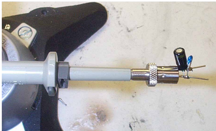
Figure 31 – Oscilloscope Probe with Probe Master ( www.probemaster.com ) 4987A BNC Adapter. (Modified with Wires for Ripple Measurement, and Two Parallel Decoupling Capacitors Added.)
