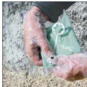
Automatic and leakproof opening of the pouch through installation of the filling nozzle.
