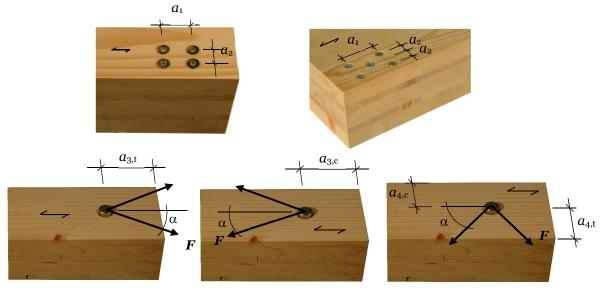
Definition of spacing, end and edge distances in the edge surface unless otherwise specified in the technical specification (ETA or hEN) for the cross laminated timber.
