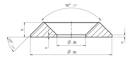
Washer for Power-Fast and construction screws
