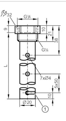
1 fixing bracket for centring piece
