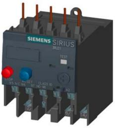
OVERLOAD RELAY 0.90...1.25 A FOR MOTOR PROTECTION SZ S00, CLASS 10, F. MOUNTING ONTO CONTACTOR MAIN CIRCUIT: RING CABLE LUG AUX. CIRCUIT: RING CABLE LUG MANUAL-AUTOMATIC-RESET
