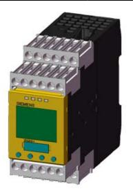
SIRIUS SAFETY RELAY SAFETY-RELATED SPEED MONITORING, 24 V DC, 45.0 MM, SCREW TERMINAL, FK INSTANTANEOUS.: 2NO, FK DELAYED: 0, MK: 2 ELECTRICAL, AUTO START / MANUAL START, BASIC UNIT, MAX. ERR. CAT. EN13849-1: E, MAX. ERR. SIL TO IEC61508:3,
