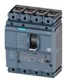
CIRCUIT BREAKER 3VA2 IEC FRAME 160 BREAKING CAPACITY CLASS L ICU=150KA @ 415 V 4POLE, LINE PROTECTION ETU320, LI, IN=25A OVERLOAD PROTECTION IR=10A ...25A SHORT CIRCUIT PROTECTION II=12 X IN NEUTRAL PROTECTION ADJUSTABLE(OFF,100%) CABLE CONNECTION
