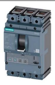
CIRCUIT BREAKER 3VA2 IEC FRAME 160 BREAKING CAPACITY CLASS M ICU=55KA @ 415 V 3POLE, LINE PROTECTION ETU330, LIG, IN=40A OVERLOAD PROTECTION IR=16A ...40A SHORT CIRCUIT PROTECTION II=1,5...12 X IN GROUNDFAULTPROTECTION IG=0,2... 1 X IN, TG=0,1/0,3MS CABLE CONNECTION
