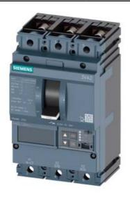
CIRCUIT BREAKER 3VA2 IEC FRAME 250 BREAKING CAPACITY CLASS M ICU=55KA @ 415 V 3POLE, LINE PROTECTION ETU560, LSIG, IN=250A OVERLOAD PROTECTION IR=100A ...250A SHORT CIRCUIT PROTECTION ISD=0,6..10X IN, II=1,5..10X IN NEUTRAL PROTECTION OPTIONAL WITH EXT. CT,UPTO 160% GROUNDFAULT, SWITCHABLE IG=0,2... 1 X IN, TG=0,050,8MS BUSBAR CONNECTION
