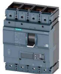
CIRCUIT BREAKER 3VA2 IEC FRAME 630 BREAKING CAPACITY CLASS C ICU=110KA @ 415 V 4-POLE, LINE PROTECTION ETU860, LSIG, IN=400A OVERLOAD PROTECTION IR=160A ...400A SHORT CIRCUIT PROTECTION ISD=0,6..10X IN, II=1,5..15X IN NEUTRAL PROTECTION ADJUSTABLE (OFF, UPTO 160%) GROUND-FAULT, SWITCHABLE IG=0,2... 1 X IN, TG=0,05-0,8MS BUSBAR CONNECTION
