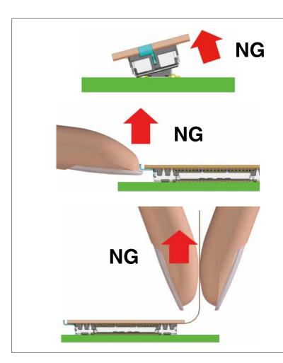
Caution! If unmated forcefully, the connector may be damaged.
