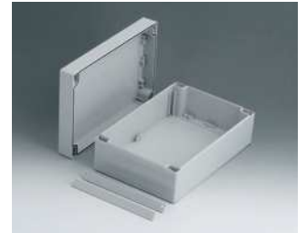
C2116242 ROBUST-BOX 160 BREIT, Ausf. II PC (UL 94 HB) lichtgrau RAL 7035 240x160x90mm IP 66
