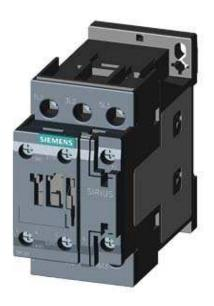
CONTACTOR, AC-3, 15KW/400V, 1NO+1NC, AC 230V 50/60HZ, 3-POLE, SZ SO SCREW TERMINAL
